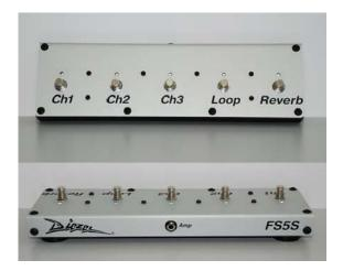
The footswitch controls all channels, the loop and the reverb.
